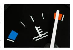
gauge on the left side of the dash. This gauge monitors the temperature of the engine.
